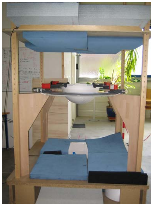
Fig 6. Measurement setup for UHF labels
